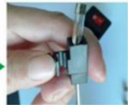
3. Remove the damaged fuse with a screwdriver
