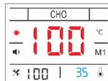
Due to the material of the hot plate and environmental factors, when the temperature is set to 100°C the temperature above the hot plate is measured to 95°C with a thermometer. In the temperature measurement calibration interface, enter the value 95°C, and press
